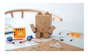
A robot recommended for beginners of programming, assembled from pieces of cardboard and controlled by tablet or a smartphone app.
