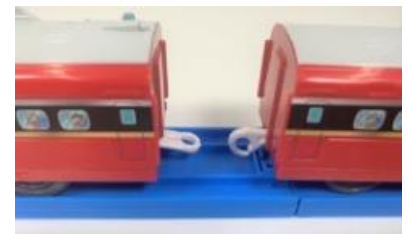
Connector part for normal PLARAIL cars. Ring and hook connector parts are used.
