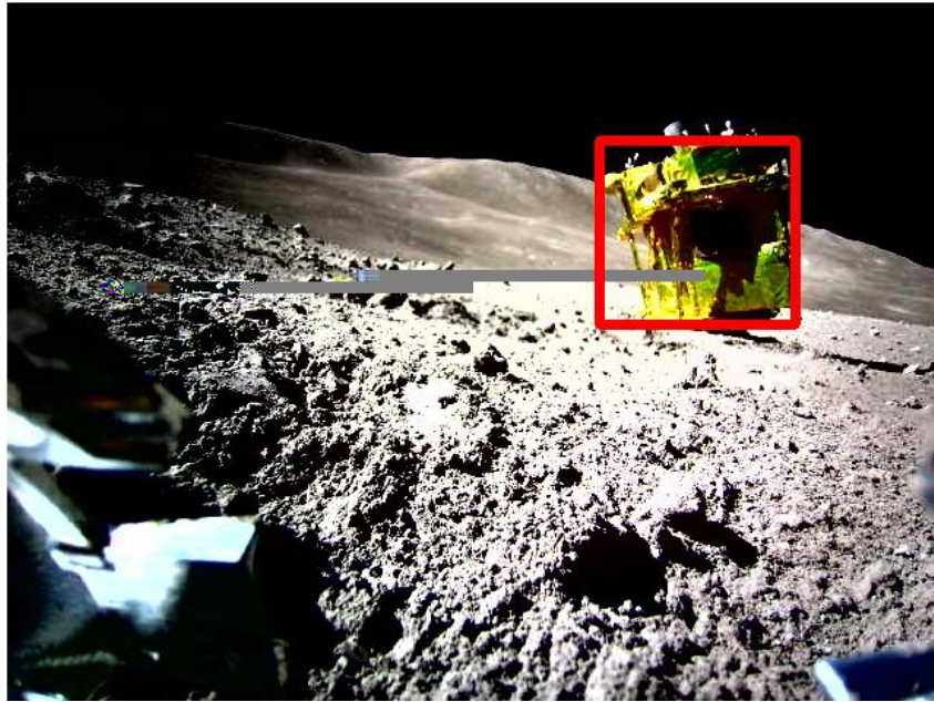
Figure 1: Lunar surface image captured by the front camera of LEV-2. (Red box indicates the detected lander on the lunar surface, demonstrating that the onboard image processing algorithm functioned correctly under lunar conditions.)
