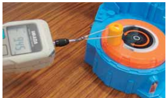
Product strength testing (TOMY checks more than 500 different safety and quality inspection items for each TOMICA)
