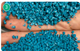
Crushed runner material (top) and normal product (bottom)
